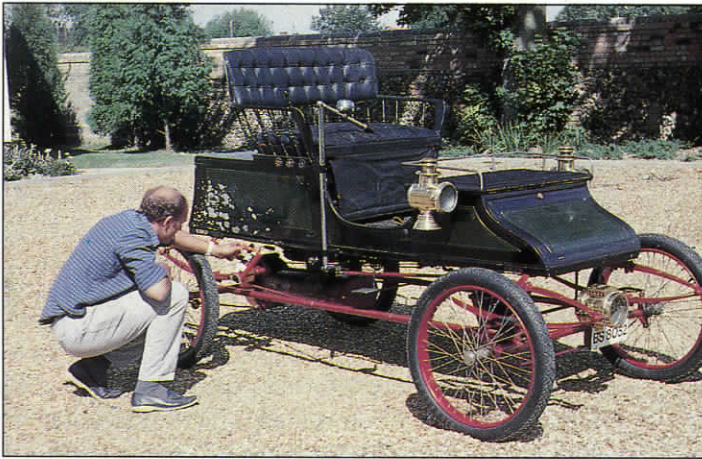
Above: Pre-heating the pilot light before the main burner can be lit to raise steam.
